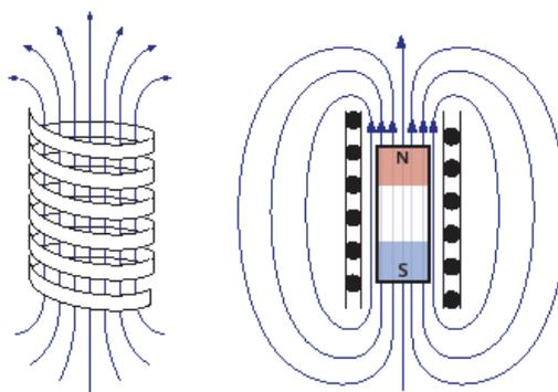
Figure 5. (left) Magnetic field alignment inside the coil of a speaker. (right) Cross-section showing magnet in field.
