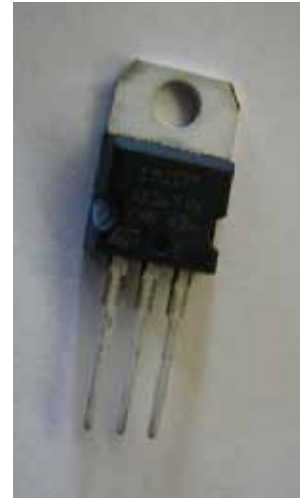
Figure 2 - LM317 three terminal adjustable regulator
